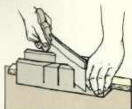
1 Cut off the waste
