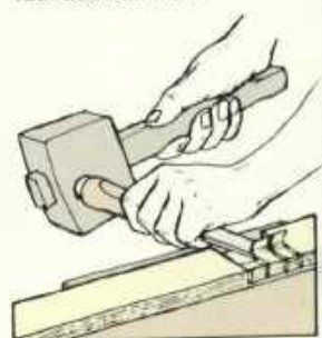
5 Chisel out the waste
